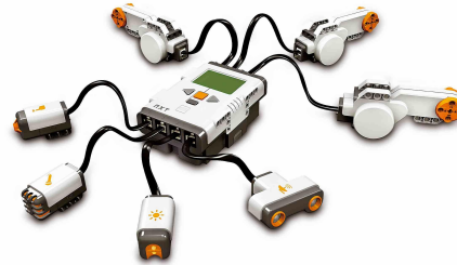
Figure 8. A NXT with 4 input sensors (touch, sound, light and ultrasonic). The 3 motors are also shown.
