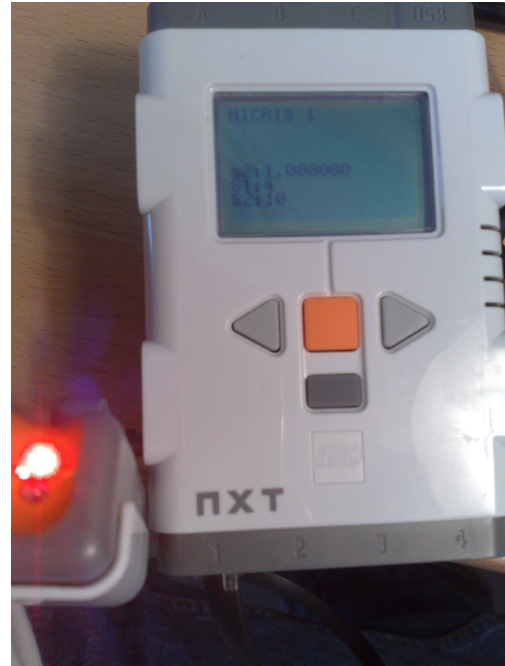
Figure 3. Micro Information System (MICRIS). Developed using Lego Mindstorms NXT. See the two Sourceforge projects nxtgcc and the nxtsquawk project at dev.java.net . It is developed using the Eclipse nescdt editor plugin for TinyOS. The text on the first line on the display is MICRIS 1.
